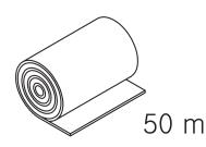
Adhesive metal strip The adhesive metal strip MKB can be used, for example, to secure covers on cable trays indoors. The adhesive tape is an alternative to turning bolts and can be applied without drilling or other tools. Butt joints can also be sealed with the adhesive tape. It is made of aluminium, is 50 mm wide and 50 m long.
