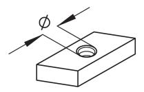
AM 12 channel nuts are threaded plates used with profile rails B 3 and B 6. The threaded hole is centred by turning the nut 90° after inserting or tipping in the nut. Channel nuts, also known as locking plates, are primarily used for spaced mounting in conjunction with long bolts or threaded rods. They are made of hot-dip galvanised steel with M6 or M8 threads and stainless steel with M8 threads.
