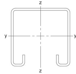
$$\begin{aligned}W_y &= 2,01 \text{ cm}^3 \\W_z &= 2,91 \text{ cm}^3 \\I_y &= 4,19 \text{ cm}^4 \\I_z &= 5,96 \text{ cm}^4\end{aligned}$$
