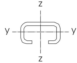
$$\begin{aligned}W_y &= 0.29 \text{ cm}^3 \\W_z &= 0.80 \text{ cm}^3 \\I_y &= 0.21 \text{ cm}^4 \\I_z &= 1.12 \text{ cm}^4\end{aligned}$$
